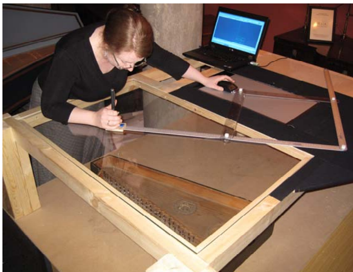
Pantograph built as part of the 'Drawing to Scale' project being used to document an octave spinet by Poggi/Orlandus (4311)
